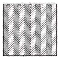
1 Thoroughly clean the floor and open different packages. Keep the left and right-hand boards well separated, and lay them ready with the groove on the long side facing you.
