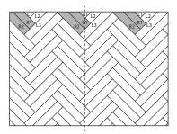
1 Thoroughly clean the floor and open different packages. Keep the left and right-hand boards well separated, and install them ready with the groove on the long side facing you.
